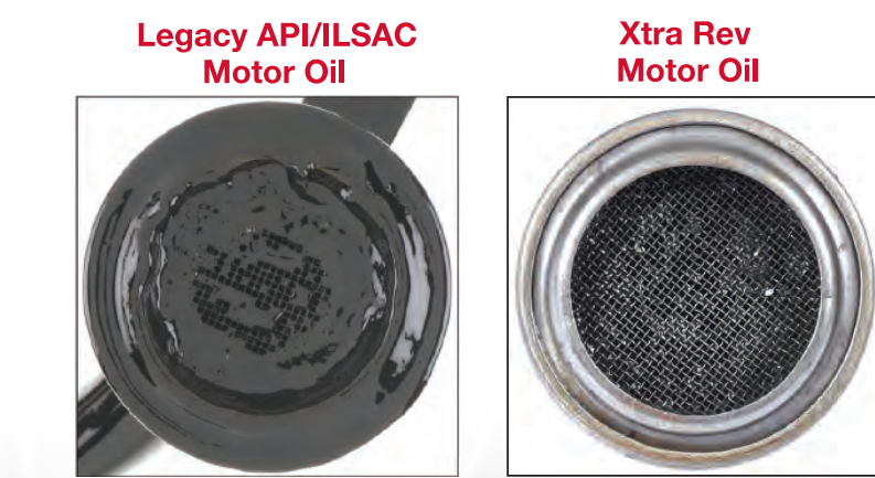
Oil screen attached to pick-up tube
