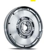
LuK engineered and developed the dual-mass flywheel to absorb engine vibrations before they are transmitted to the driveline. When torque spikes occur, the DMF allows the primary section of the flywheel to turn independently from the secondary section, saving the driveline and transmission from damage.
