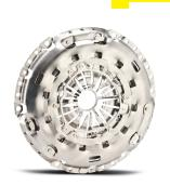
The Self Adjusting Clutch was designed and patented by LuK to keep pedal effort low over the life of the clutch. In addition to increasing driver comfort, the SAC design extends the life of the clutch.
